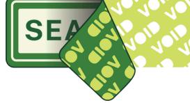
a memory card compartment door. Staff can easily spot evidence of tampering or unauthorized access by comparing seal numbers to logs and/or by spotting voided seals.
